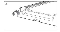
b. If the walking belt has shifted to the right, first remove the key and UNPLUG THE POWER CORD. Using the allen wrench, turn the left adjustment bolt counterclockwise 1/4 of a turn. Plug in the power cord, insert the key and run the treadmill for a few minutes. Repeat until the walking belt is centered.
